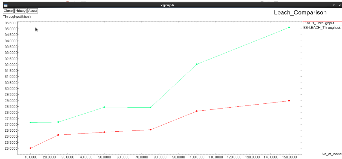
Figure 8: the Throughput Demonstrating the Efficiency of the Network between Leach and IEE-LEACH
